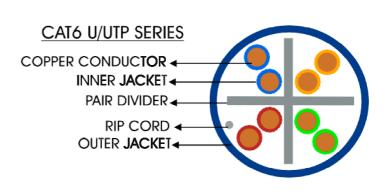
CAT6 cables reduce crosstalk and system noise. The superior insulation around the 23AWG copper wires attributes to the increase performance. They cable transmit data at 1000Mbps (1Gigabit per second) with a frequency of 250MHz and suitable for 10BASE -T, 100BASETX fast ethernet and 1000BASE-T / 1000BASE-TX (Gigabit Ethernet)
